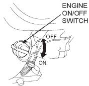
Figure 12. Engine ON/Off Switch
